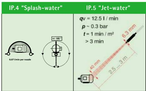
Protection degree IP.5 is an important requirement for the often requested suitability of chemical plants for "Outdoor Installation", however a number of supporting constructional and production engineering measures as well as an endurance test are necessary.
